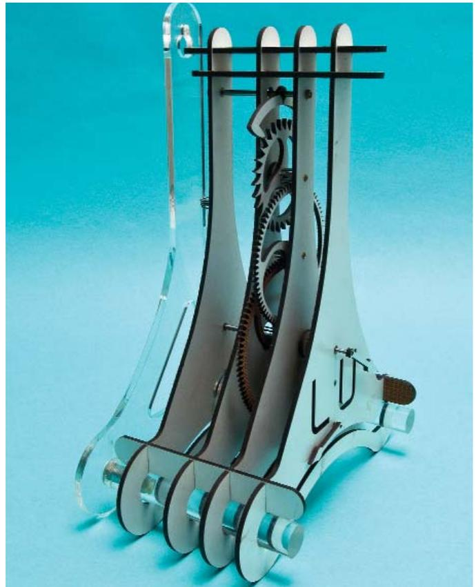
4. Fibreglass construction with lantern pinions.
